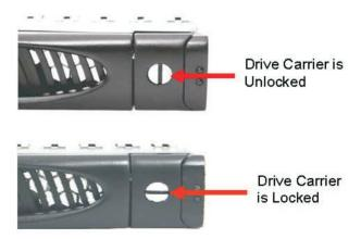
2. The Lock Grooves are located on a button. Press the button and the Drive Tray handle will flip open.
