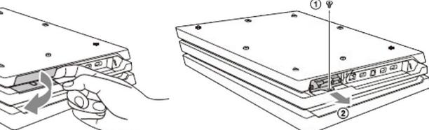
4. Once you reveal the HDD bay, use a screwdriver to remove the screw.
