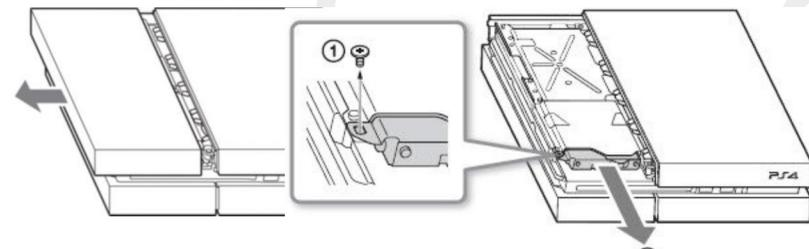
5. Remove the four screws that anchors the HDD and remove the HDD.
