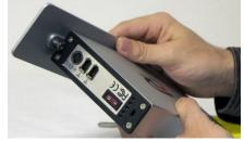
4. Once the foot is fully inserted into the groove, tighten the screws at the bottom of the base with the Philips screwdriver by turning them clockwise.
