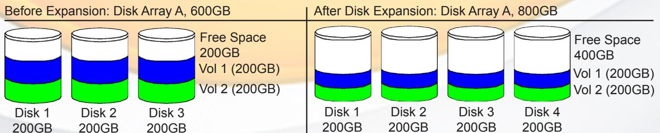
The RAIDBank4 controller redistributes the original volume set over the original and newly added disks, using the same fault-tolerance configuration. The unused capacity on the expanded RAID set can then be used to create additional volume sets, with a different fault tolerance setting if required.
