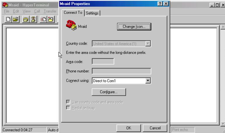
Step 8. Open the Settings Tab. Function, arrow and ctrl keys act as: Terminal Keys, Backspace key sends: Ctrl+H, Emulation: VT100, Telnet terminal: VT100, and Click OK.
