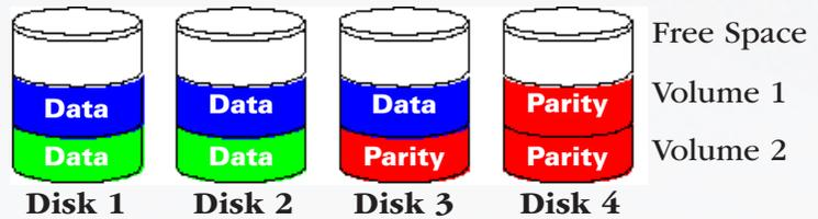
A 4 Disk RAIDset may contain two volumes. Volume 1 can be assigned a RAID 5 level of operation while Volume 2 might be assigned a RAID 0+1 level of operation.
