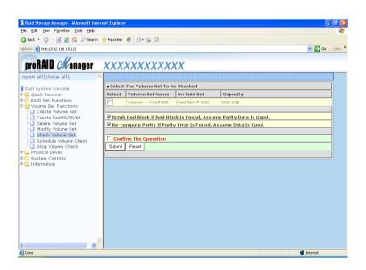
Use this option to verify the correctness pf the redundant data in a volume set. For example, in a system with dedicated parity, volume set check means computing the parity of the data disk drives and comparing the results to the contents of the dedicated parity disk drive. The checking percentage can also be viewed by clicking on RaidSet Hierarchy in the main menu.
