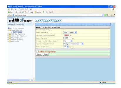
The number of physical drives in the raid subsystem determines the RAID levels that can be implemented with the raid set. You can create a raid set associated with exactly one volume set. The user can change the raid level, capacity, Volume Initialization Mode and stripe size . A hot spare option is also created depending upon the existing configuration.
