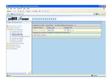
Migrating occurs when a disk is added to a raid set. Migration status is displayed in the raid status area of the Raid Set information when a disk is added to a raid set. Migrating status is also displayed in the associated volume status area of the volume set Information when a disk is added to a raid set.
