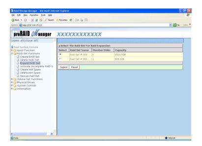
To expand a raid set, click on the **Expand Raid Set** link. Select the target raid set, which you want to expand it.
