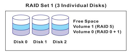
tion and data on that raid set. If a server fails to work, the raid set disk drives can be moved to another server and inserted in any order.
